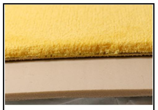
Thickness: .250 (1/4") Density per cu. ft. 16 lbs, Width: 6 Ft or 12 Ft. Standard Roll Length: 100 FT
